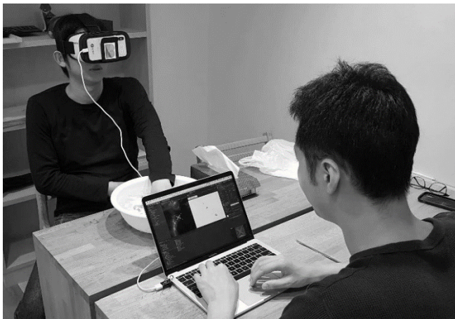
Fig. 4. Experiment setup including Smartphone based VR-HMD, controller PC, water with ice in wash ball.
